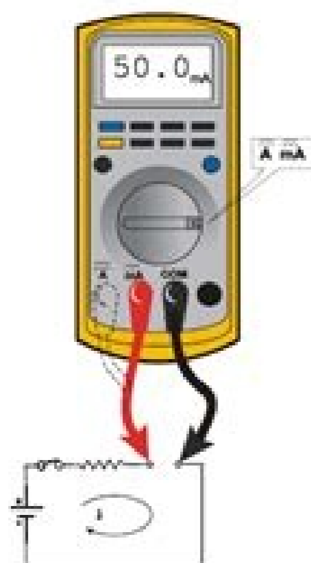
Figure 7-4. Current Measurement (DC)
